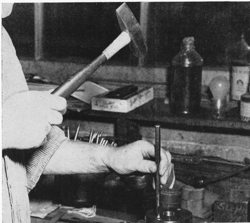
What's wrong? No, it's not the bandaged hammer, that's just the way a craftsman in a machine room identifies his own. Wrong, however, is the use of a hard steel hammer against a hard drift also hitting against a hardened piece of work. This causes pieces to chip off, dangerous pieces. One should always use a soft-headed hammer against a hard drift against soft work, never hard against hard as staged above.
